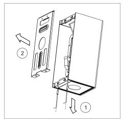
take off the mounting bracket by Allen-key screw driver.
