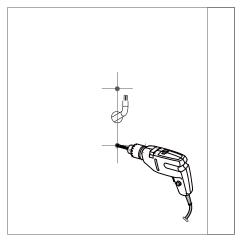
3. Drill two holes on the wall (Ф=8mm, depth=50mm, distance 85-125mm)
