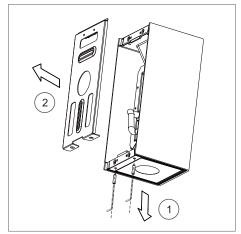
1. take off the mounting bracket by Allen-key screw driver.
