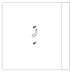
4. Fix the expansion bolt into the holes
