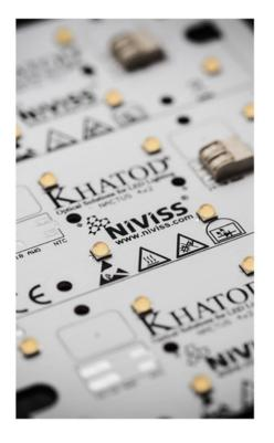
Niviss modules are also characterized by a long life thanks to the use of some of the best diodes on the market and thermal optimization, which we are able to simulate for the customer using specialized software.
